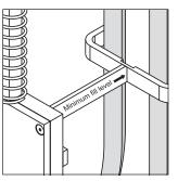
Keep the magazine filled to the "minimum fill line".
