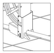
Place the tool over the PEX tubing and a mesh wire parallel to the tubing.
