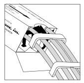
Load directly from the clip box to the magazine. See the PEX-2-Mesh Clips<sup>™</sup> box for details.
