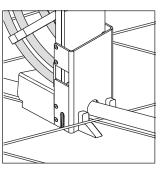
Using your foot, slide front forks under the mesh then depress the handle firmly until the clip locks the tube to the wire.
